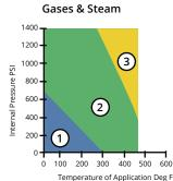
The pressure/temperature graphs shown are the most current method of determining the suitability of a gasket material in a known environment. Use the pressure and temperature graphs to select the most suitable material for your application.
