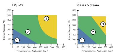
The pressure/temperature graphs shown are the most current method of determining the suitability of a gasket material in a known environment. Use the pressure and temperature graphs to select the most suitable material for your application.
