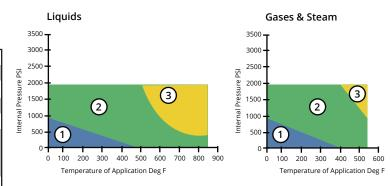
The pressure/temperature graphs shown are the most current method of determining the suitability of a gasket material in a known environment. Use the pressure and temperature graphs to select the most suitable material for your application.
